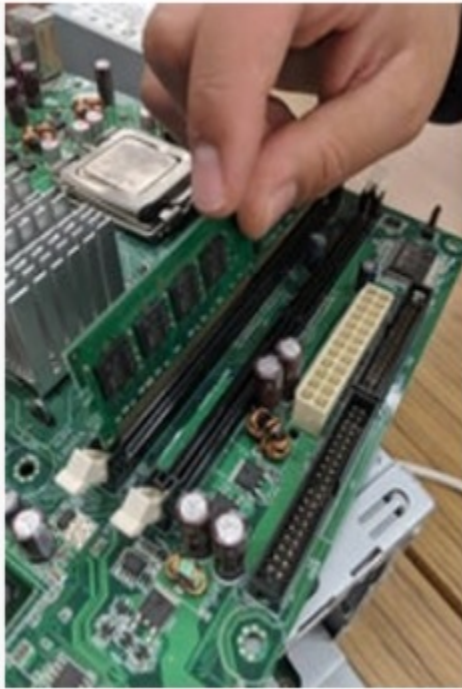
Figure 9.6 Remove RAM chips
