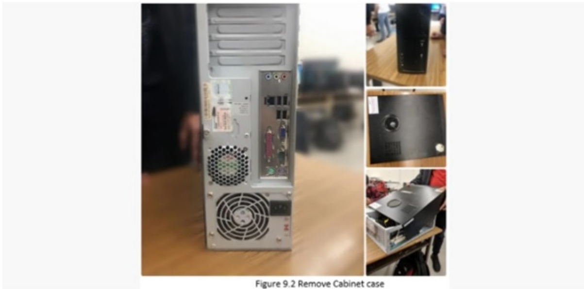
Figure 9.2 Remove Cabinet case
