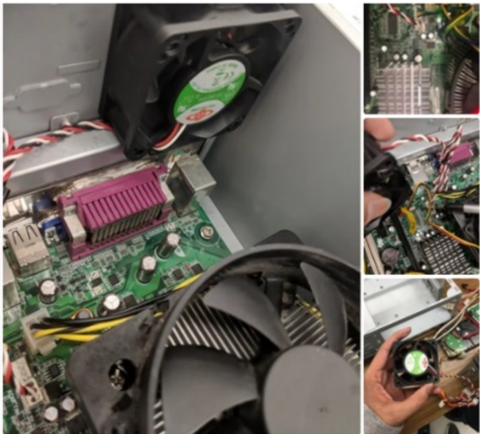
Figure 9.5 Remove System FAN
